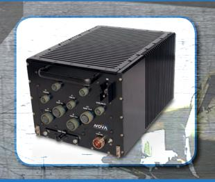
The 3000 Series consists of a family of standard products and custom ATR reference designs also referred to as a chassis or enclosure. They support highly rugged and MIL-spec applications utilized by the defense and aerospace markets. The Series provides a full set of packaging features ideally suited to meet the high performance demands of ground-based applications or flight vehicles that operate at high altitudes.
