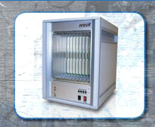
NIS's small footprint, instrumentation-style enclosure is a development chassis with 42HP internal width accommodating up to ten (10) 3U x 160mm boards on 4HP centers (0.8 inch) or eight (8) boards on 5HP centers (1.0 inch). A typical VPX configuration consist of a 6 slot backplane on 5HP centers and a single plug in power supply. A rear transistion card cage can also be installed which is accessible via a rear opening, hinged door, or custom I/O panel.
