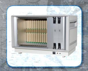
NIS's small footprint, instrumentation-style enclosure is a development chassis with 42HP internal width accommodating up to twenty (20) 3U x 160mm boards on 4HP centers (0.8 inch) or sixteen (16) boards on 5HP centers (1.0 inch). A typical VPX configuration consist of a 12 slot backplane on 5HP centers and dual plug in power supplies. A rear transistion card cage can also be installed which is accessible via a rear opening, hinged door, or custom I/O panel.
