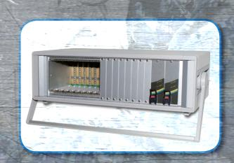
NIS's small footprint, instrumentation-style enclosure is a development chassis with 42HP internal width accommodating up to ten (21) 3U x 160mm boards on 4HP centers (0.8 inch) or sixteen (16) boards on 5HP centers (1.0 inch). A typical VPX configuration consist of a 12 slot backplane on 5HP centers and dual plug in power supply. One or two PICMG 2.11 hot swap/redundant/N+1 plug-in power supplies can also be accommodated, with either AC or DC input.
