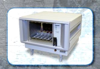
NIS's small footprint, instrumentation-style enclosure is a development chassis with 42HP internal width accommodating up to ten (10) 3U x 160mm boards on 4HP centers (0.8 inch) or eight (8) boards on 5HP centers (1.0 inch). A typical VPX configuration consist of a 6 slot backplane on 5HP centers and a single plug in power supply. One or two PICMG 2.11 hot swap/redundant/N+1 plug-in power supplies can also be accommodated, with either AC or DC input.
